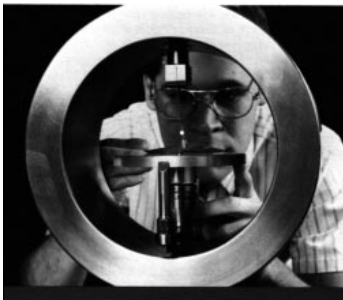
Fig. 1. CCRL inspector uses elastic calibration device (called a proving ring) to verify loading accuracy of a laboratory testing machine.
