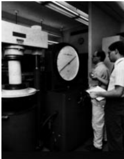
Fig. 2. CCRL inspector evaluates laboratory technician's procedure during routine compressive strength test of cylindrical concrete specimen.
